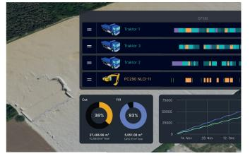
Using the Dashboard data, our Simulation tool allows digital rehearsals to happen in the virtual space, where different combinations of equipment and soil distributions can be tested out before they start happening onsite.
